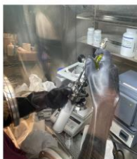
LiCl-KCl salt prep in Ar glove box
